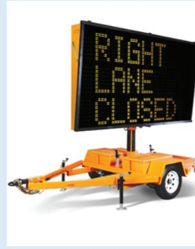
These systems enable construction crews to program and place a message at needed locations without the hassle of refueling generators. Solar array and battery banks are typically sized to enable the signs to operate for several days even in poor weather conditions.
