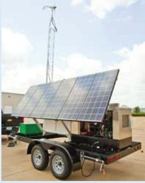
These include small power systems mounted on a trailer frame with two or more independent power sources to provide reliable, self-sustained power for diverse applications and environments. They may require no refueling and offer silent operation for deploying sensors, camera and antennas in security, remote power, disaster relief, emergency preparedness, and lighting applications.
